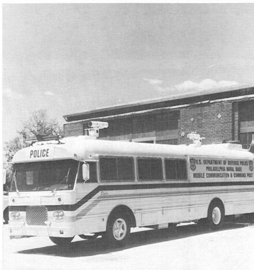
Philadelphia's Mobile Communication and Command Post bus is equipped with a 12-person conference center and a communication room with police, fire, ambulance, military, shipboard and aircraft radio equipment, cellular telephones and two roof-mounted high-powered video cameras for viewing and recording accident and disaster scenes. (Photo by John Long)
