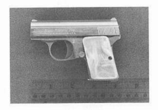
Another firearm of similar concern due to its concealability is the Bauer Stainless Steel Auto. This single action, semi-automatic also has an overall length of four inches but weighs ten ounces. It is manufactured in .25 caliber and has a magazine capacity of six rounds with a seventh round available in the chamber. This pistol is manufactured by the Bauer Firearms Corporation and is a copy of the "Baby Browning," which can no longer be imported to the United States due to
