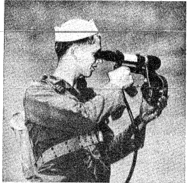
Sniperscope shoots out an infra-red beam which illuminates the target and reflects the target image in the rifle telescope.
